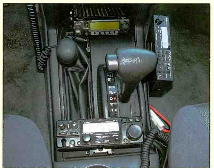
This is a direct overhead shot of the gear and console area. The ICOM 2-meter rig is at the top of the picture, the PRO-2026 is to the right of the console (heavy duty fasteners are great, aren’t they?), and the Alinco HF rig is at the bottom. The CB set (a small RS unit that was on sale about four months ago) has been removed pending installation of a Midland 75-822 CB set, which saves even more space.
