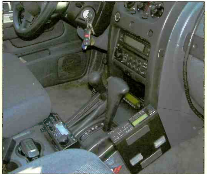
This is a shot from the passenger’s side of the cab after I had cleaned up the installation, routed and dressed the wires and coaxial cable, and added the Alinco DX-70T HF rig (rear of center console). Notice how nice things look now. The spiral wrap coming down on the right side of the dash has both speaker wires along with the in/out for the HF SWR/power meter.
