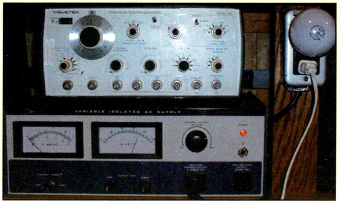
Photo G. My dim-bulb tester is permanently mounted on the bench adjacent to the Heath SP-5220 variable, isolated AC supply. The dim-bulb tester is made from an odd combination of socket and AC plug on a single electrical plate.
