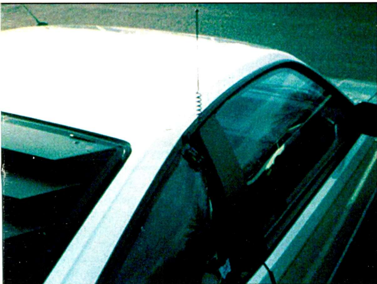
Typical on-glass mobile cellular antenna installation on the CRX.
