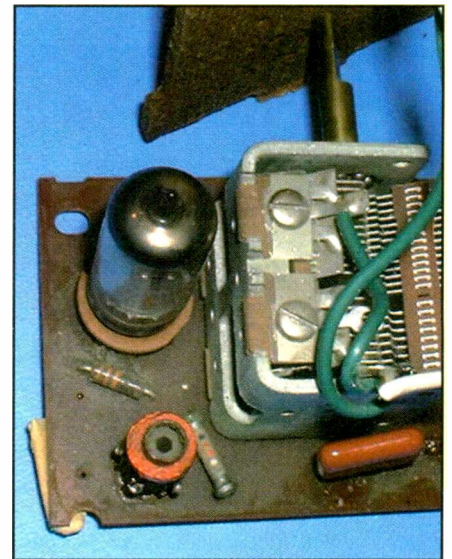
Photo H. Alignment points: The C1-A-T (antenna trimmer) and C1-B-T (oscillator trimmer) 2-14-pF mica trimmers can be seen on the top frame of the tuning capacitor. The oscillator trimmer is towards the front (control side) of the board.
