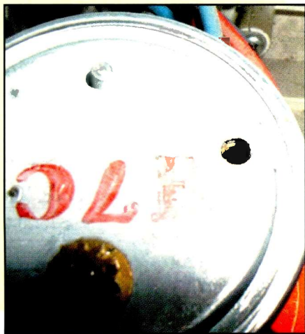
Photo J. A small hole is drilled in the front plate of the gearbox so fresh clock oil can be added to the mechanism. Care must be taken to prevent drill chaff from entering the gearbox, where it could bind the gears or cause premature wear. I smashed a plastic gear when the drill entered too far into the opening.
