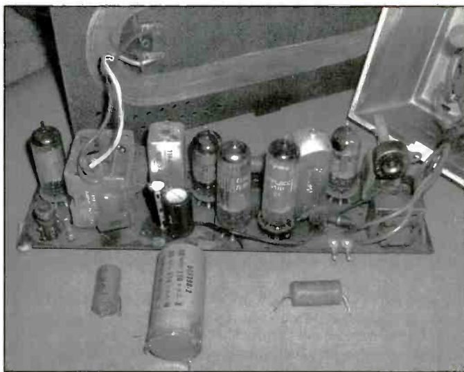
Photo B. Top view of the pc board. The replaced capacitors, two wax paper caps, and dual-section filter are shown in the foreground. The two replacement radial-lead electrolytic caps can be seen on the rear of the board.
