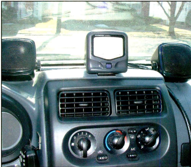
Here's a look at the dual speakers (one for the HF rig and the other for the 2-meter rig) that I found at RadioShack on sale for about $10 for the pair! In the middle is the Diamond cross-needle SWR/Power meter for the HF station. This type of unit is small, saving space, and nice to have to accurately tune the motorized antenna on the rear of the truck.
