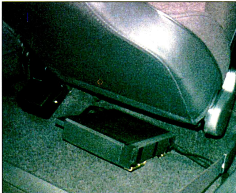
Here’s a professional-grade cellular mobile phone transceiver box.
