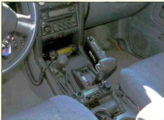
Here is a console shot from the driver’s side after the clean up. The rig in the center of the dash is the ICOM IC-2100H 2-meter transceiver. To the right, on end, attached to the side panel of the console with Velcro is my old RadioShack PRO-2026 VHF/UHF scanner. The Alinco DX-70T HF rig is below the shift lever. Actually, that is only the control head, the actual radio sits under the passenger’s seat. The mic for the HF rig, along with the antenna tuning control, sits in the cup holder in the console.
