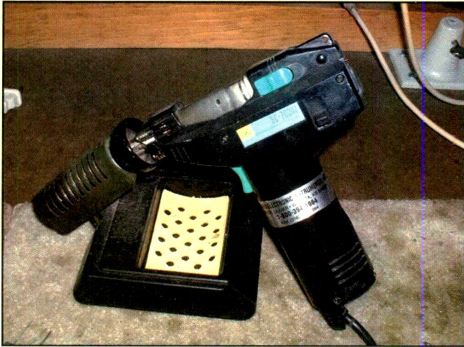
Photo F. Albeit expensive, this Denon SG-7000Z handheld desoldering tool is the professional approach to pc board desoldering.
